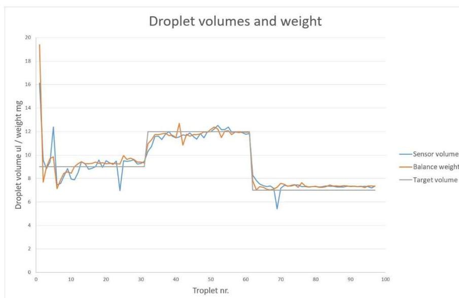
Figure 3: a control loop adjusts the plunger stroke to follow the targeted volumes.
